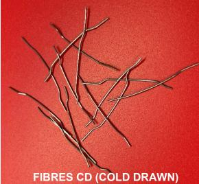
Cold drawn process gives a tensile strength 3 times higher than the melt extracted technique
